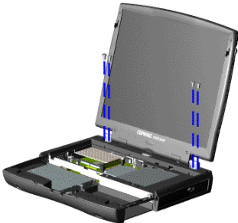
10. Support the back of the display panel assembly and remove two screws from each of the display panel hinges.
