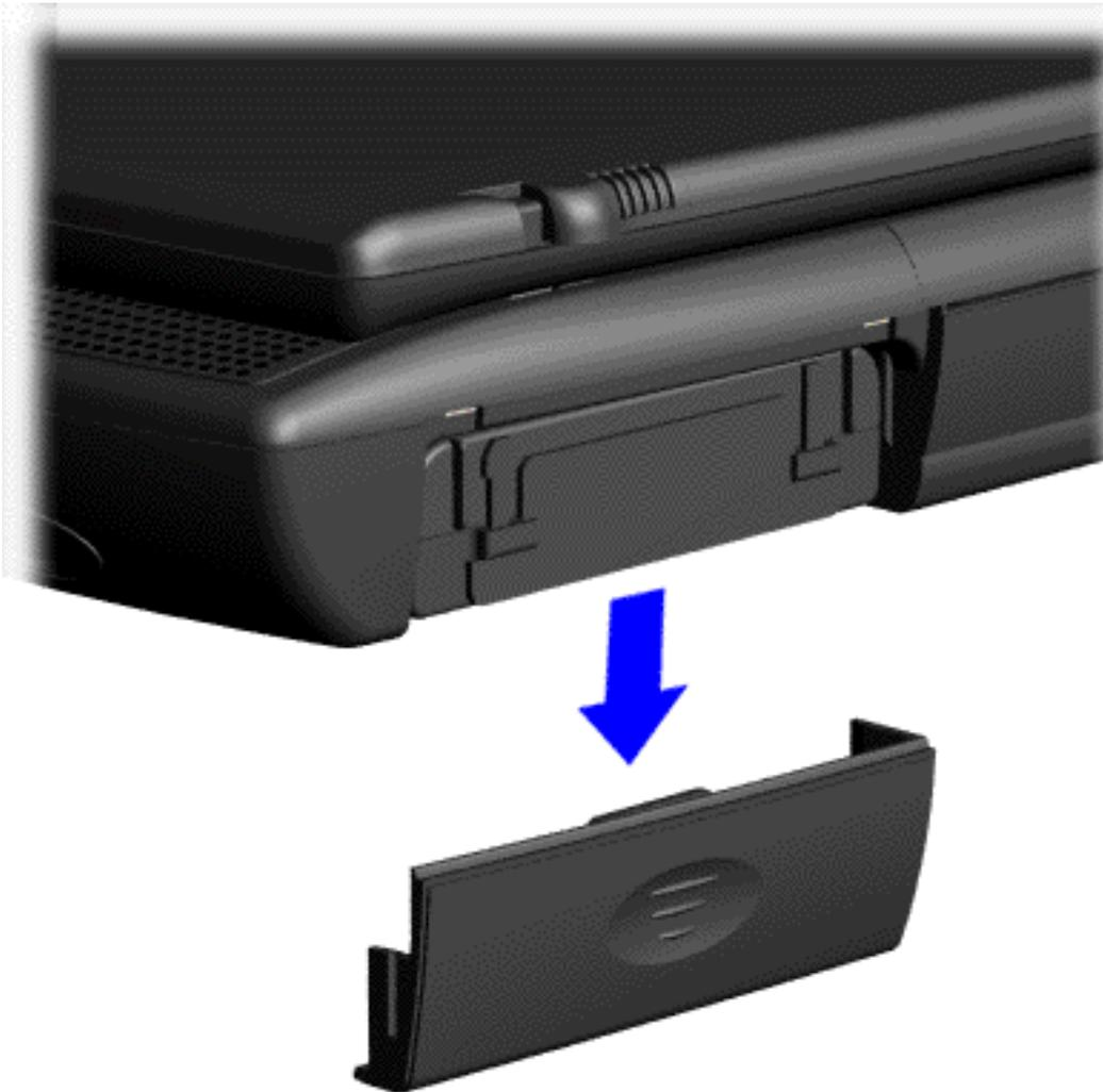
To remove the battery pack, complete the following steps:
