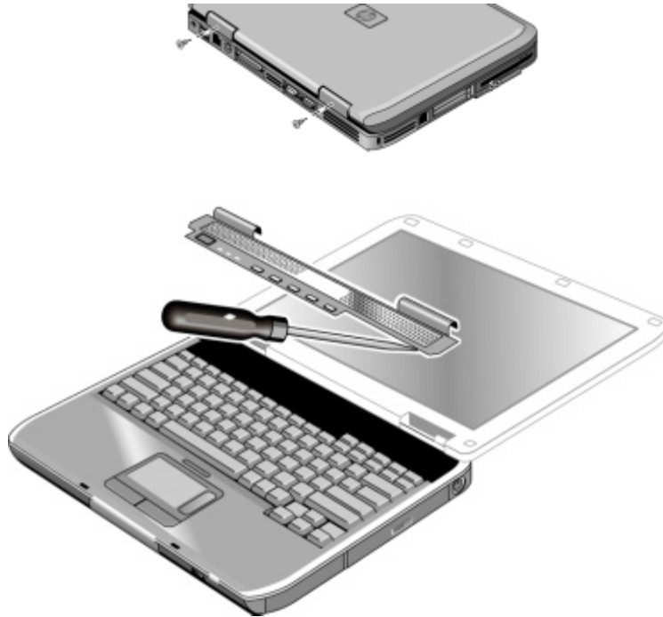
Figure 2-9. Removing the Keyboard Cover
