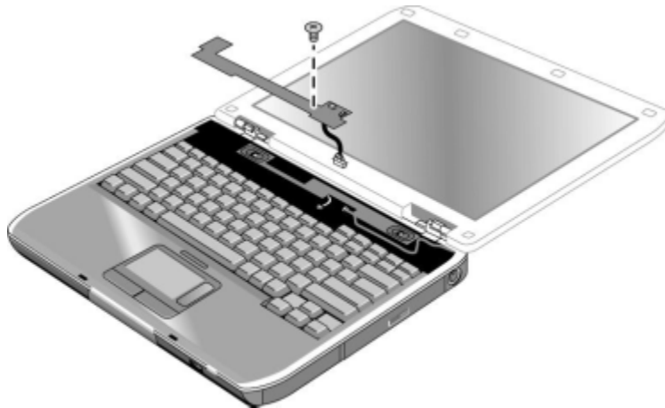
Figure 2-13. Removing the Switchboard PCA
